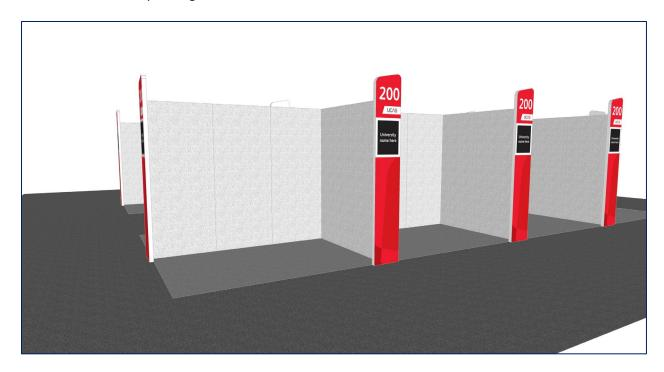
The shell scheme panels are finished in high quality, fire retardant, nylon loop material, and are manufactured to comply with Class 1 fire regulations. They allow for the easy fixing of display items using Velcro tapes and tabs. The walls are butt jointed panelling, 2.44m high and 50mm thick, and are pre-finished in nylon loop material. Please note that 25 – 50mm may be lost from the width of your
